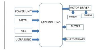
The proposed Arduino-based robotic system provides several advantages tailored to the unique demands of the electrical field. By integrating a metal sensor, gas sensor, ultrasonic sensor, buzzer, and Wi-Fi module, this robot is specifically designed to operate safely and efficiently in narrow and hazardous electrical environments. Key advantages of this proposed system.
